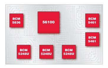
The **BCM56100** is the fifth generation of the highly-integrated and costeffective Broadcom StrataSwitch and StrataXGS product line in a singlechip solution, with twenty-four FE ports and two GbE ports.
