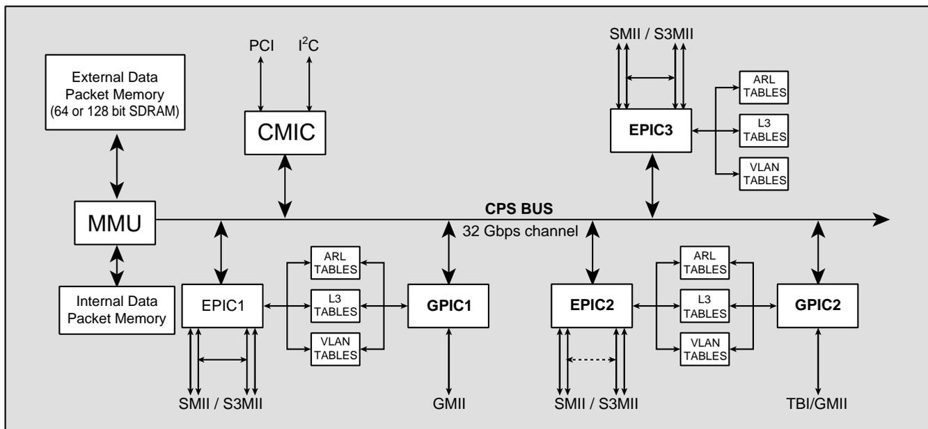
The **BCM5616**, with a forwarding rate of 6.6 Mpps, defines the next generation of performance for single-chip switching solutions. Through its advanced ContentAware™ feature set, the StrataSwitch II product family supports advanced applications and services, at wire speed, with non-blocking performance.
