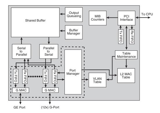
The BCM5631 switching processor chip supports 12-Gigabit ports with all ports in wirespeed operation. The BCM5631 is ideal for applications such as multi-Gigabit port switches or aggregating multiple-Gigabit ports.
