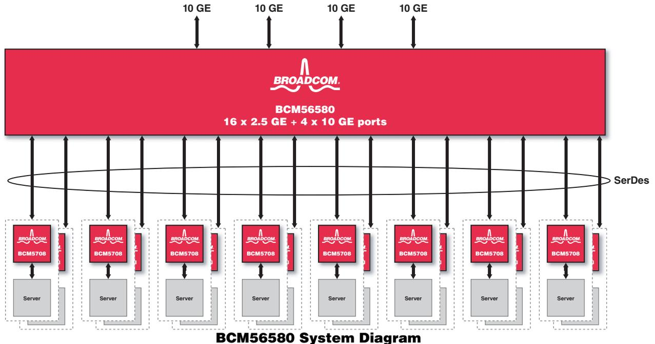
The BCM56580 network switch is a high-density, 2.5-Gigabit Ethernet switching chip solution with 20 ports. Additionally, the BCM56580 integrates all the SerDes required to interface to applicable copper and fiber physical interfaces. The integrated SerDes functionality includes 10-Gbps XAUI interfaces and 2.5/1-Gbps SGMII PHY interfaces. The integrated SerDes complies with the CX-4 standard and PICMG3.1 standard, which ensures interoperability with Ethernet line cards in an advanced TCA chassis.
