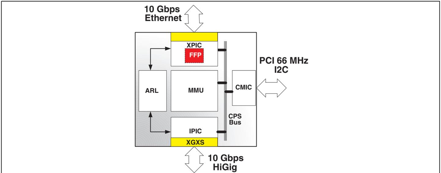
The BCM5673 10 Gigabit Ethernet switch is a scalable, multi-layer switch-on-chip member of the StrataXGS family. The BCM5673 is a dual port switch, which supports a 10 Gigabit Ethernet (IEEE802.3ae) port and a HiGig™ uplink port. The 10 Gigabit Ethernet port can be used to interface to the XENPAK module via the XAUI interface.
