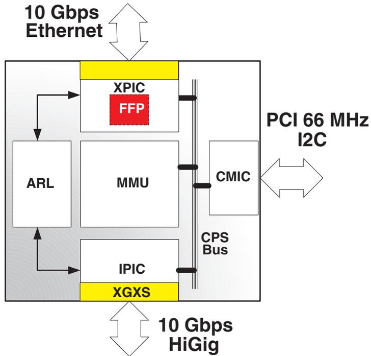
The BCM5673 10 Gigabit Ethernet switch is a scalable, multi-layer switch-on-chip member of the StrataXGS family. The BCM5673 is a dual port switch, which supports a 10 Gigabit Ethernet (IEEE802.3ae) port and a HiGig™ uplink port. The 10 Gigabit Ethernet port can be used to interface to the XENPAK module via the XAUI interface.
