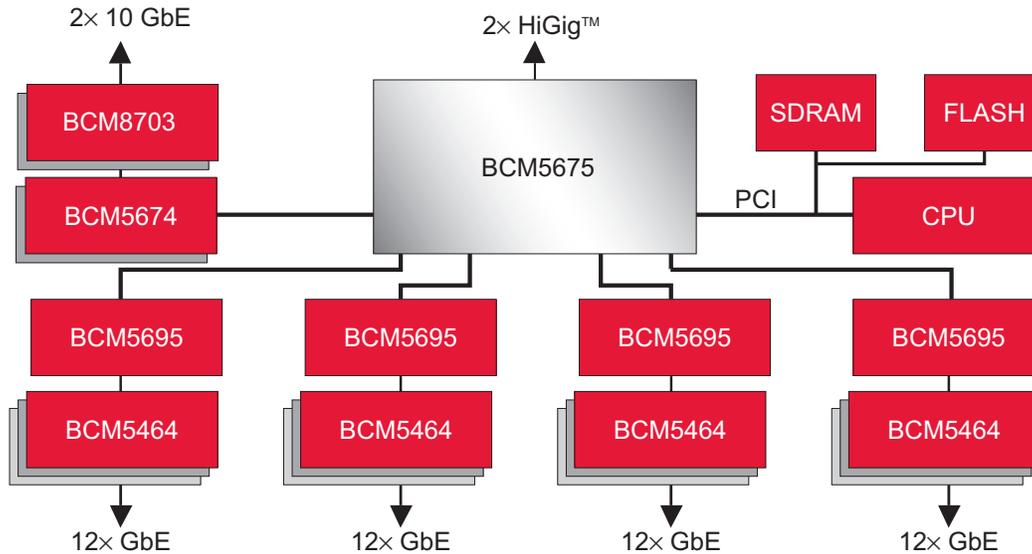
The BCM5674 10-Gigabit Ethernet switch is a scalable, multilayer switch-on-chip member of the StrataXGS family. The BCM5674 is a dual-port switch, which supports a 10 Gigabit Ethernet (IEEE 802.3ae) port and a HiGig™ uplink port. The 10 Gigabit Ethernet port can be used to interface to the XENPAK module via the XAUI interface.
