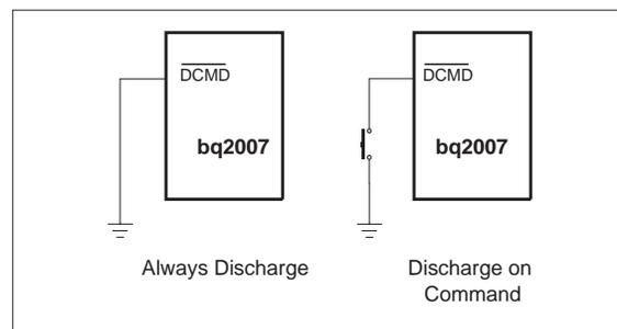
**Figure 3. Discharge-Before-Charge**
