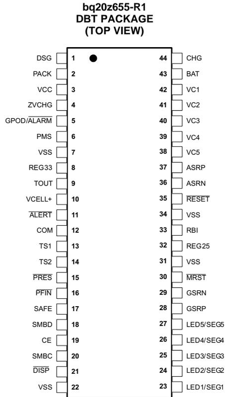
Figure 1. Package Pinout
