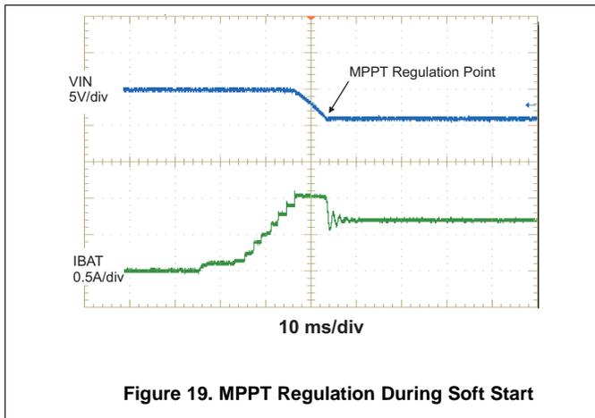
Figure 19. MPPT Regulation During Soft Start
