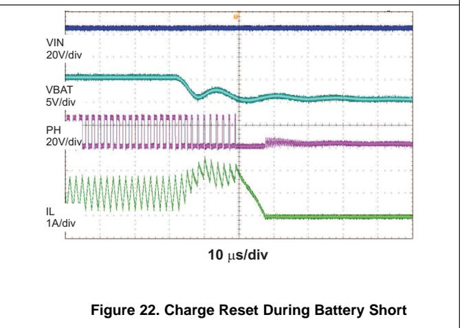
Figure 22. Charge Reset During Battery Short
