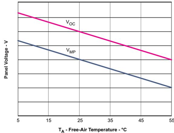
**Figure 17. Solar Panel Output Voltage Temperature Characteristics**
