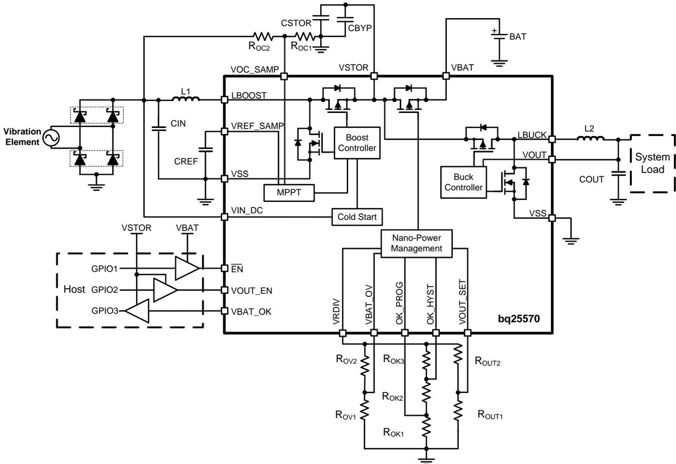
**Figure 42. Typical Externally Set MPPT Application Circuit**
