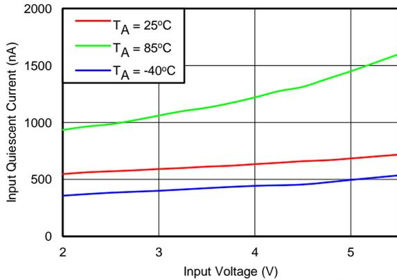
VIN\_DC = floating and  $\overline{EN}$  = GND and VOUT\_EN=VSTOR
