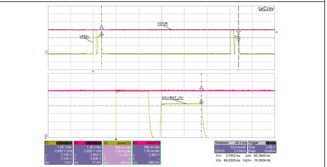
$V_{IN\_DC} =$  sourcemeter with  $V_{SOURCE} = 2.0 \text{ V}$  and compliance of  $43 \text{ mA}$
