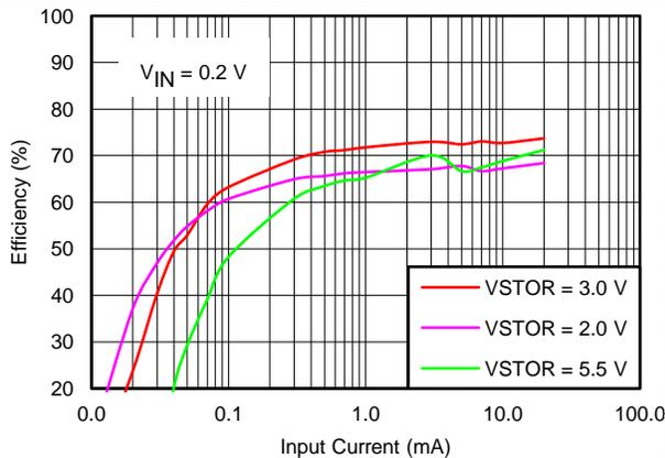
$V_{IN\_DC}$  = sourcemeter configured with voltage source = 0.2 V and  $I_{COMP}$  varied from 0.01 mA to 100 mA
