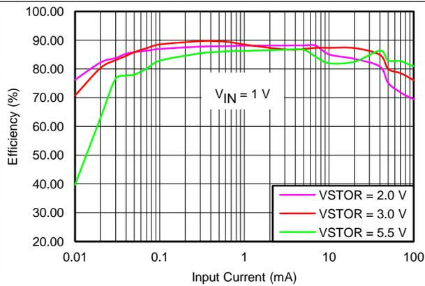
$V_{IN\_DC}$  = sourcemeter configured with voltage source = 1.0 V and  $I_{COMP}$  varied from 0.01 mA to 100 mA
