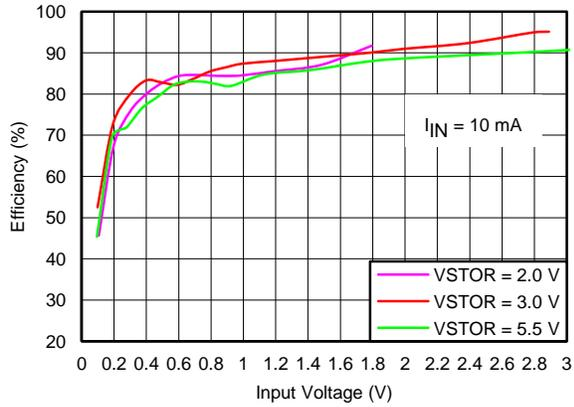
$V_{IN\_DC}$  = sourcemeter configured with  $I_{COMP} = 10$  mA and voltage source varied from 0.1 V to 3.0 V
