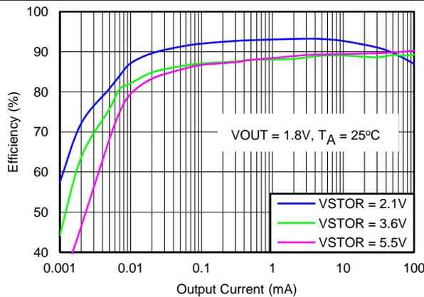
VSTOR = sourcemeter configured as a voltage source, measuring current
