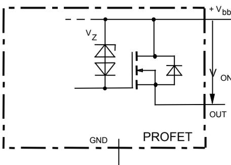
$V_{ON}$  clamped to 47 V typ.
