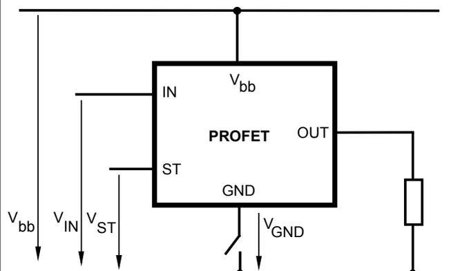
Any kind of load. In case of Input=high is  $V_{OUT} \approx V_{IN} - V_{IN(T+)}$ .
