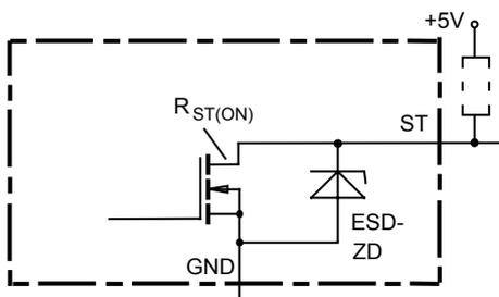
ESD-Zener diode: 6.1 V typ., max 5.0 mA;  $R_{ST(ON)} < 375 \Omega$  at 1.6 mA, ESD zener diodes are not to be used as voltage clamp at DC conditions. Operation in this mode may result in a drift of the zener voltage (increase of up to 1 V).
