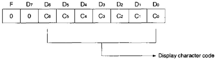
The address counter is incremented after the display data writing is complete.
