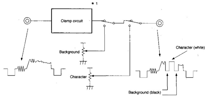
\* 1) Composite signals have their level fixed at  $1V_{P-P}$ , and the DC level is fixed. However, in many cases, the signal used has had its frequency components removed by a capacitor. To superimpose white, gray, and black levels the DC level of the signal to be superimposed must be fixed with reference to the pedestal-level voltage. This is done using a clamp circuit.
