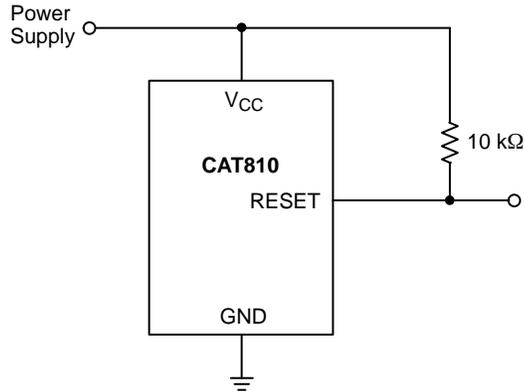
Figure 9. RESET Valid with V<sub>CC</sub> Under 1.1 V
