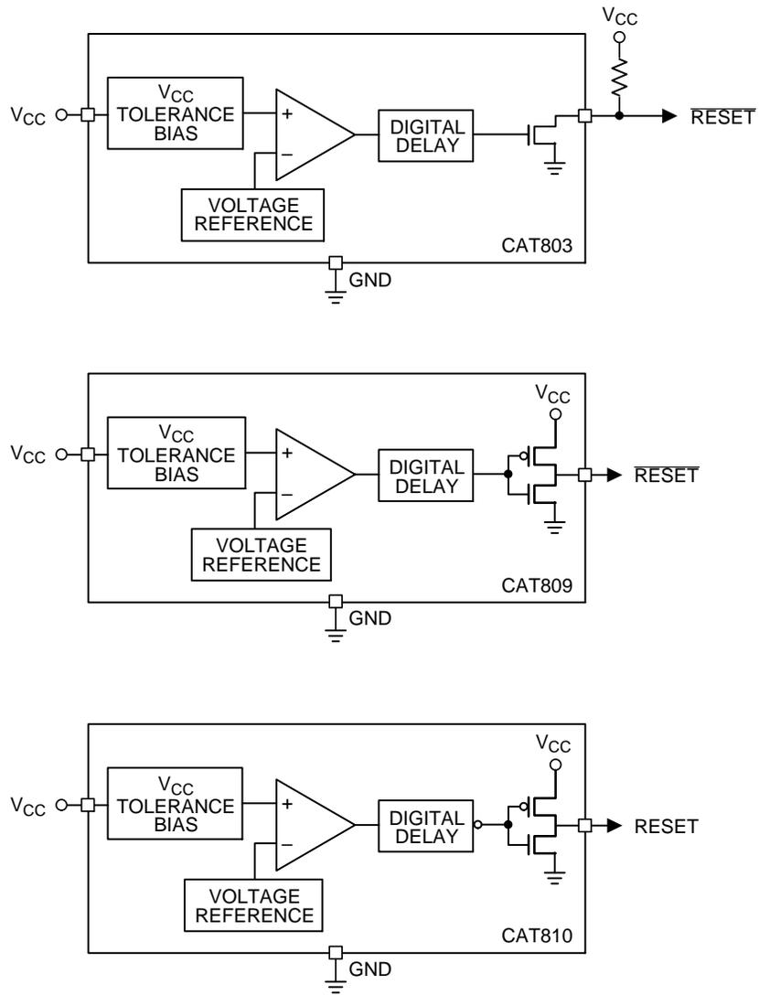
Figure 1. Block Diagrams
