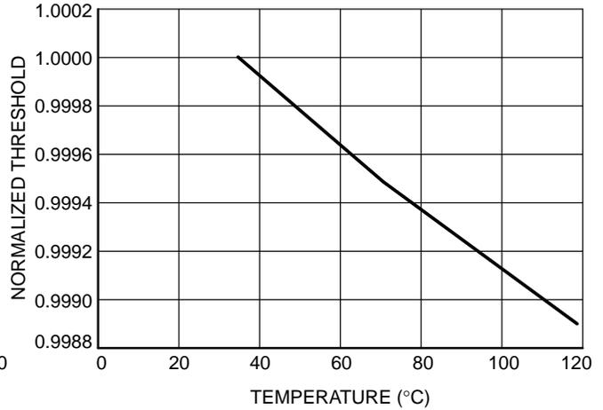
Figure 5. Normalized Reset Threshold vs. Temperature
