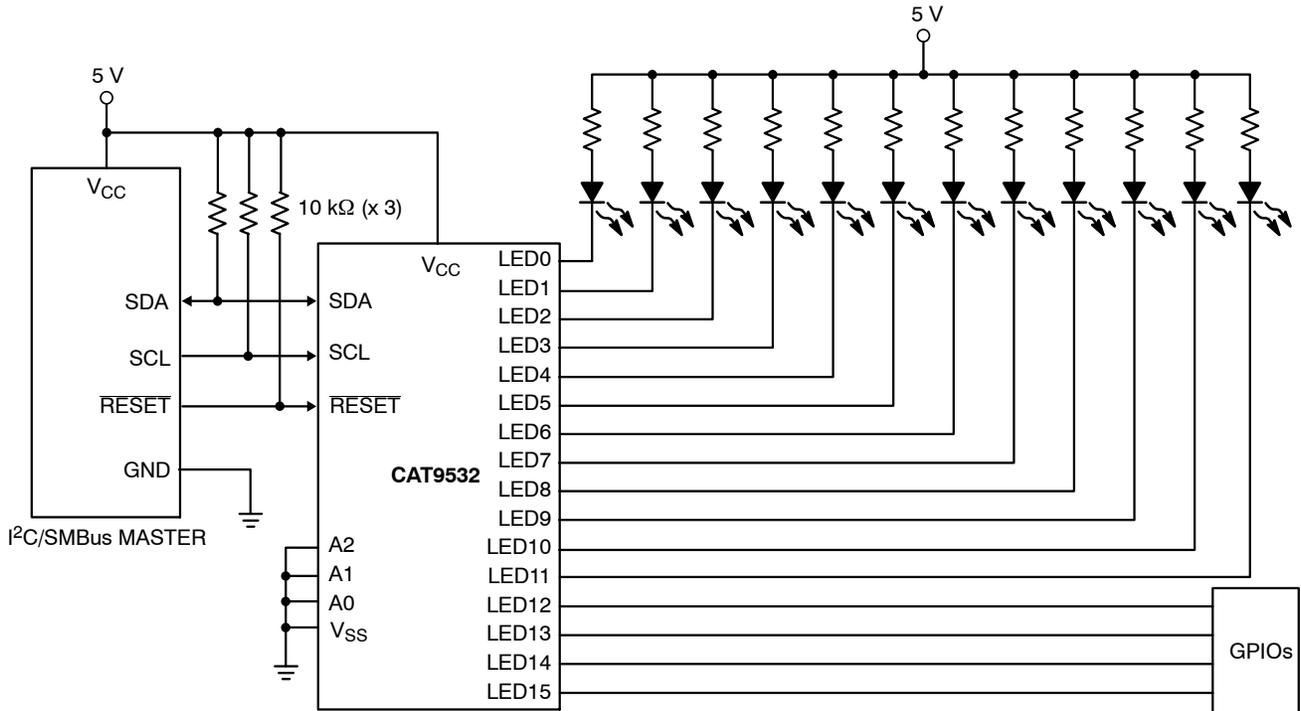
**Note:** LED0 to LED11 are used as LED drivers and LED12 to LED15 are used as regular GPIOs.
