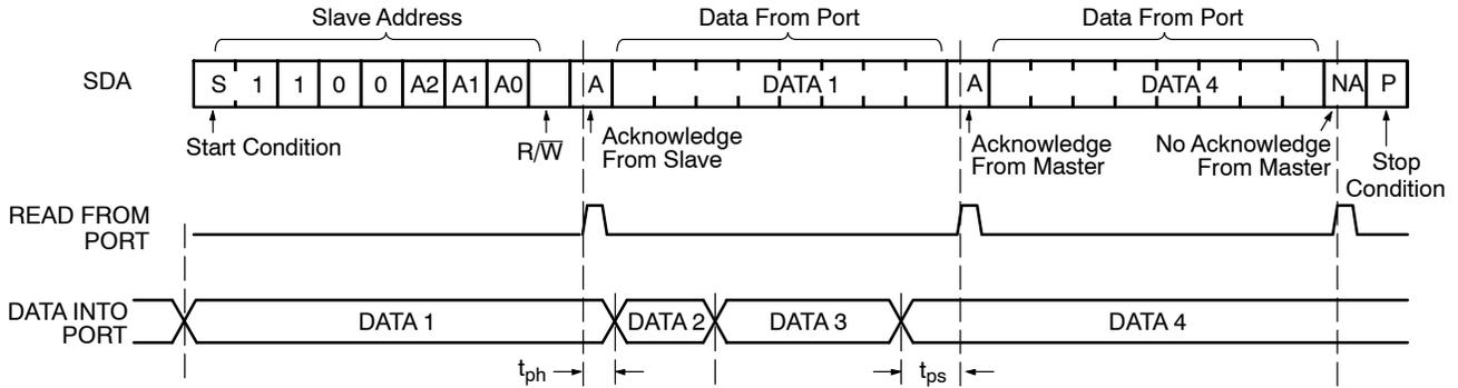
Figure 11. Read Input Port Register Timing Diagram
