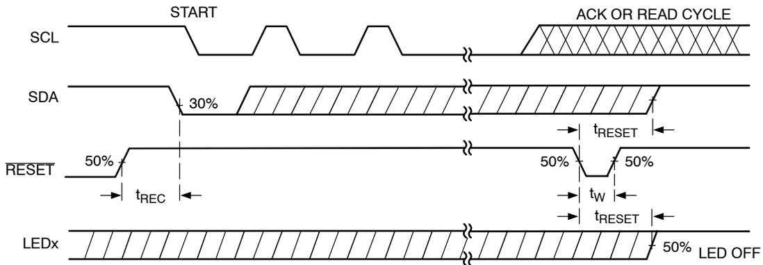
Figure 12. RESET Timing Diagram
