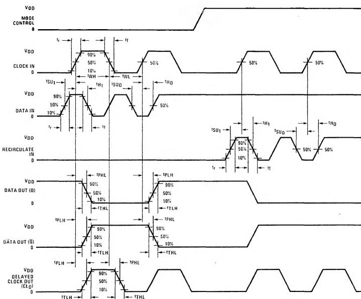
**AC Electrical Characteristics**  $T_A = 25^\circ\text{C}$ ,  $C_L = 50 \text{ pF}$ ,  $R_L = 200 \text{ k}$ , Input  $t_r = t_f = 20 \text{ ns}$ ,
