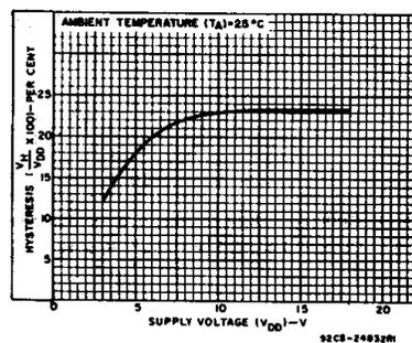
Fig. 13 – Typical per cent hysteresis vs. supply voltage.
