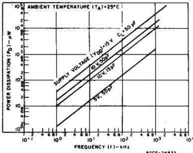
Fig. 14 - Typical power dissipation vs. frequency characteristics.
