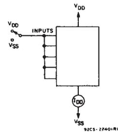
Fig. 19 - Quiescent device current test circuit.
