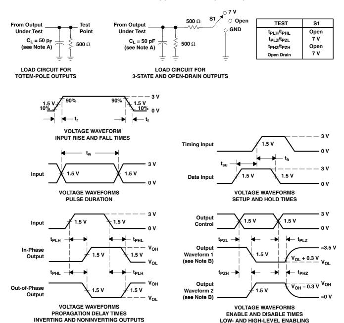
NOTES: A. C<sub>1</sub> includes probe and jig capacitance.
