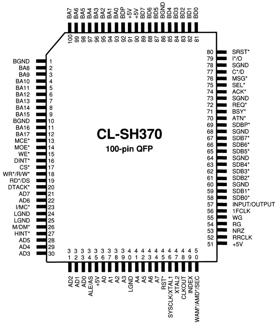
**100-pin Quad Flat Pack (QFP) Pin Diagram**
