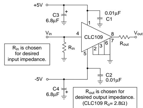
**Figure 1: Recommended circuit & evaluation board schematic**
