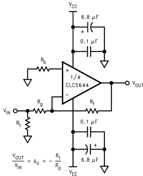
Note:  $R_b$  provides DC bias for the non-inverting input. Select  $R_t$  to yield desired  $R_{in} = R_t \parallel R_g$ .
