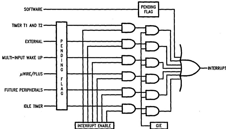
FIGURE 13. COP888CF Interrupt Block Diagram
