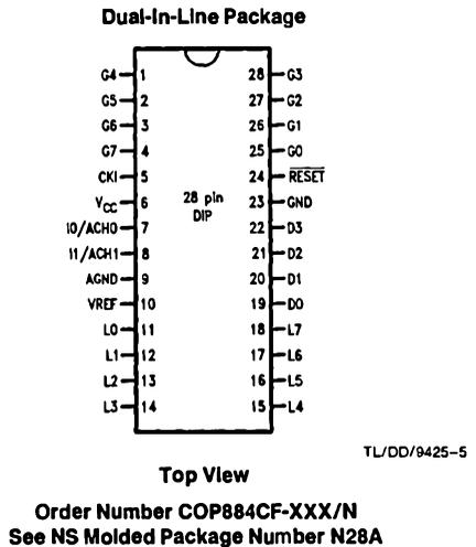
FIGURE 2. COP888CF Connection Diagrams
