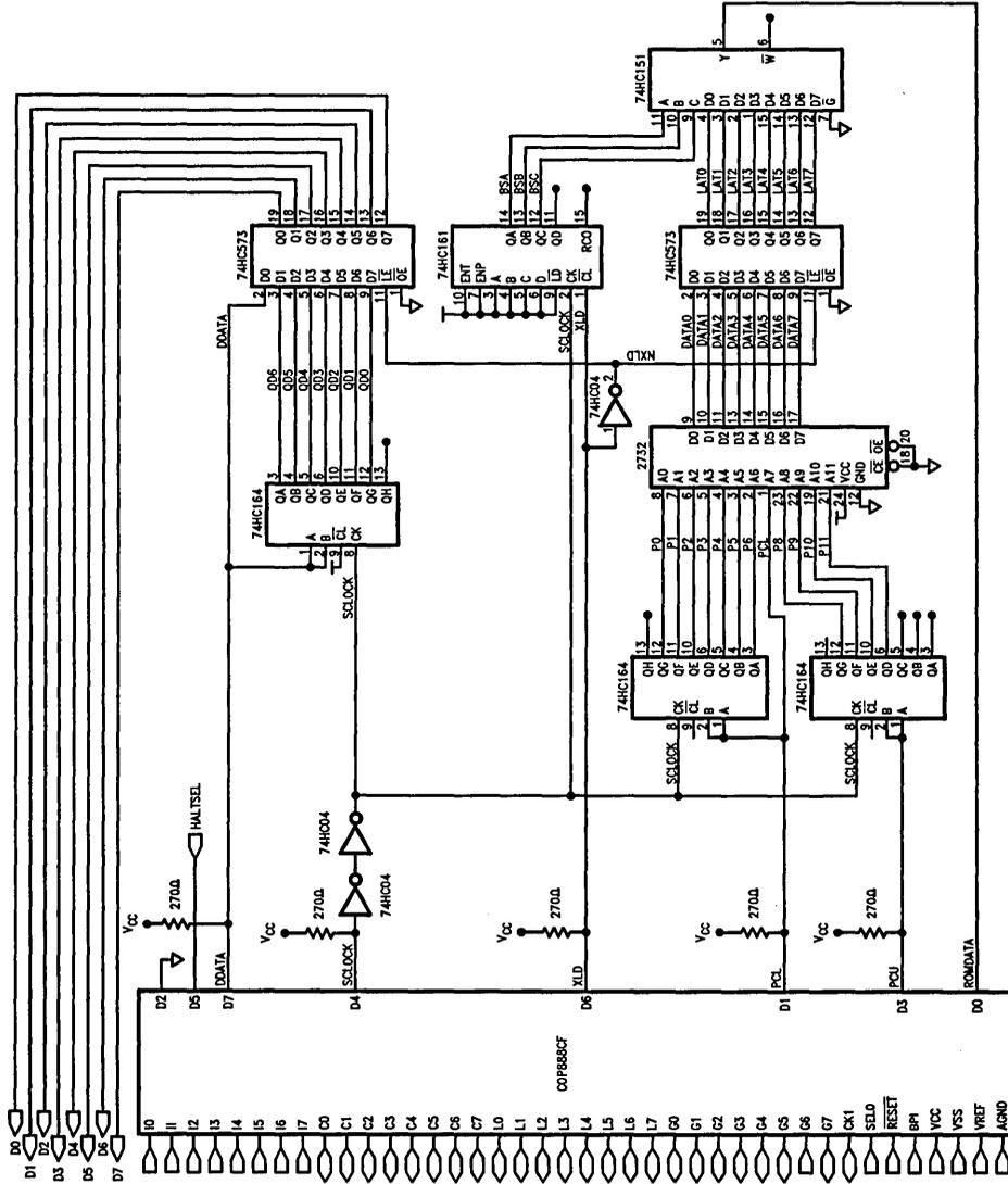
FIGURE 6. COP888CF ROMless Mode Schematic
