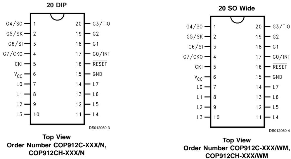
FIGURE 2. COP912C/COP912CH Pinout
