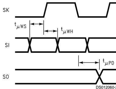
**FIGURE 1. MICROWIRE/PLUS Timing**
