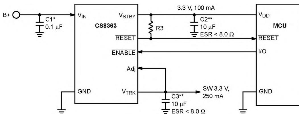
\*C1 is required if regulator is located far from power supply filter.
