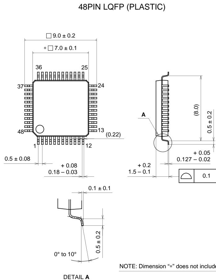
NOTE: Dimension "\*" does not include mold protrusion.
