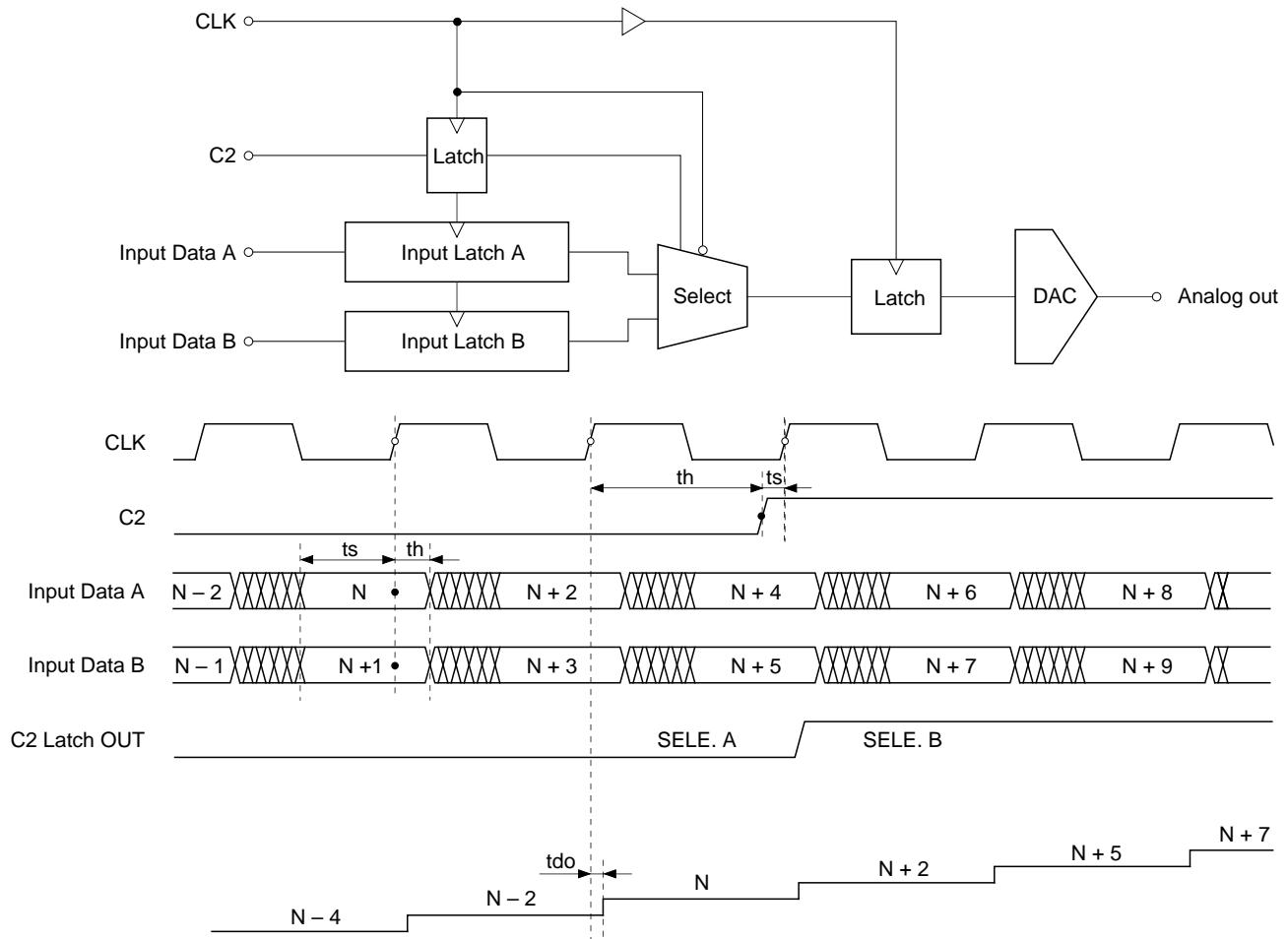
For SELE.A and SELE.B modes, input Data A or Data B is selected and the selected data can be analog output. In the state of C1=1, C3=0, Data A is selected for C2=0 and Data B is selected for C2=1.
