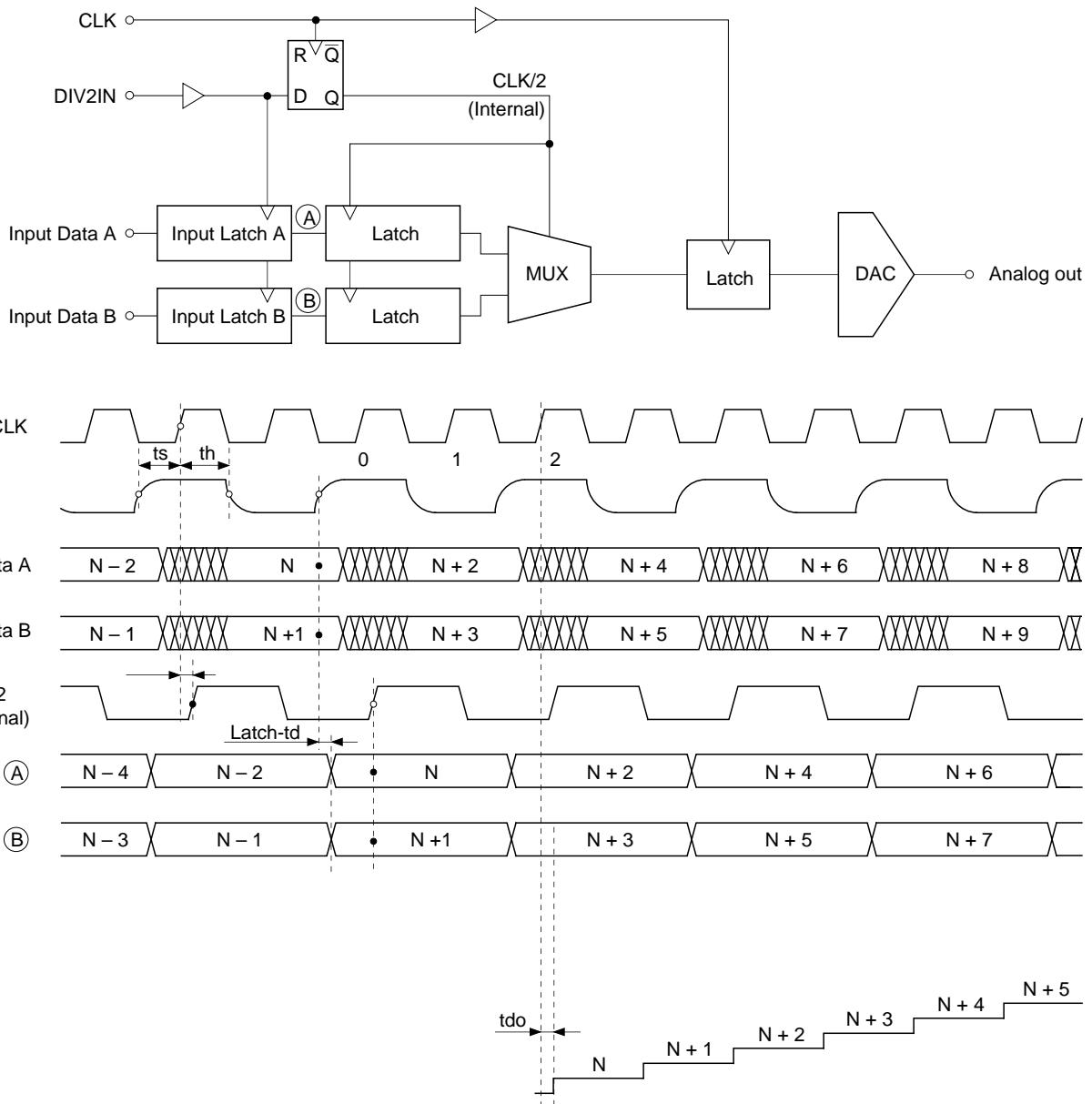
For MUX.2 mode, the frequency-halved CLK/2 and Data A and Data B, which are synchronized with CLK/2, are provided simultaneously. They are internally multiplexed and the resulting signal can be analog output.
