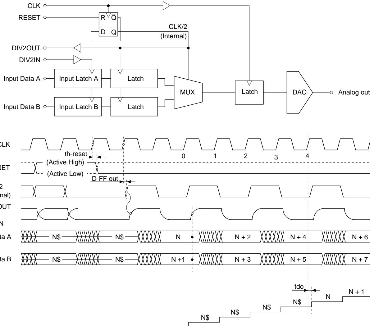
For MUX.1A mode, Data A and Data B are internally multiplexed and then the resulting signal can be analog output.
