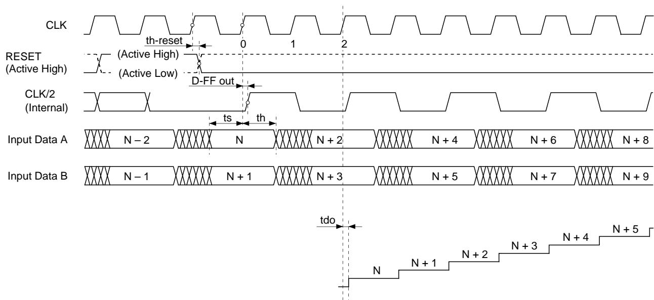
For MUX.1B mode, Data A and Data B are internally multiplexed and then the resulting signal can be analog output.
