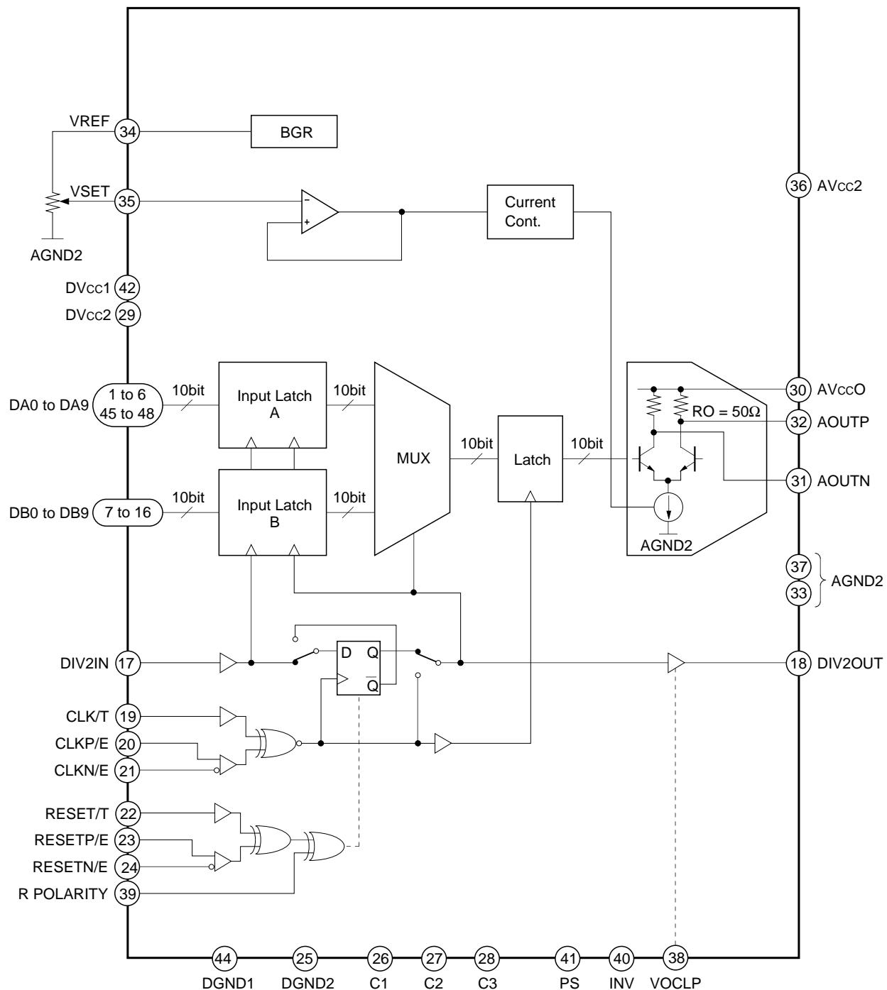
**Pin Description and I/O Pin Equivalent Circuit**
