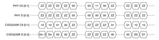
ZZ: High-impedance state, D0 to Dn: packet data
