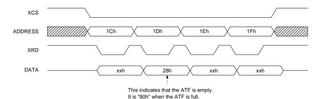
The number of quadlets that can be stored in the ATF can be found from the value of the Async Status register bits [23:19]. The following six states can be found, so a judgment must be made as to whether write is possible from the number of quadlets in the packet being sent from the external CPU.
