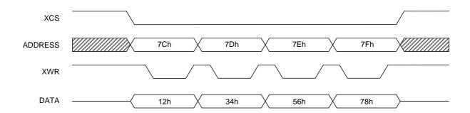
The Quadlet Write request packet is stored in the ATF as shown above. When the bus is enabled, the CXD3220R transmits automatically. If transmit does not take place, the CFR interrupt register (0Ch to 0Fh) must be read to confirm if the ATStk bit or TCErr bit is high. If these bits are high, the packet stored in the ATF may not be correct.
