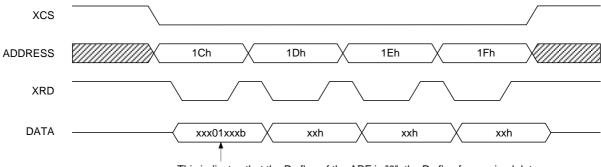
This indicates that the Dc flag of the ARF is "0", the Dc flag for received data that was read previously was not up, and that the ARF is almost empty and ATF is empty.
