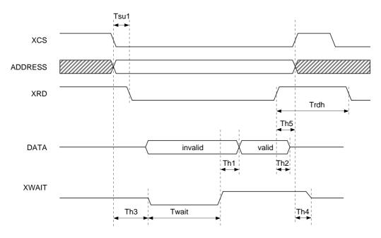
Tsu1 5nsec min, Th1 3nsec max, Trdh 60nsec min Twait 270nsec max, Th2 16nsec max, Th3 8nsec max, Th4 14nsec max, Th5 5nsec min
