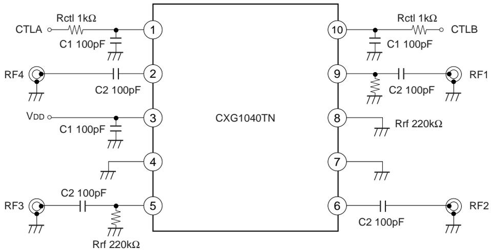
When using the CXG1040TN, the following external components should be used:
