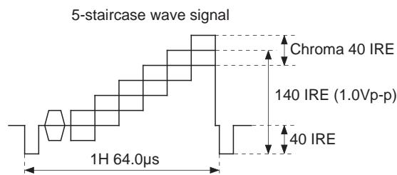
DG and DP are measured at output S point by vector scope.
