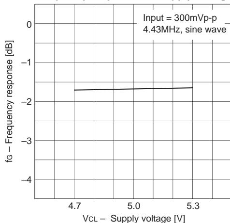
**Frequency response vs. Supply voltage**
