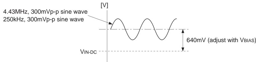
**Note 2) Differential gain and differential phase measuring condition**
