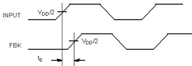
Figure 7. Device-Device Skew
