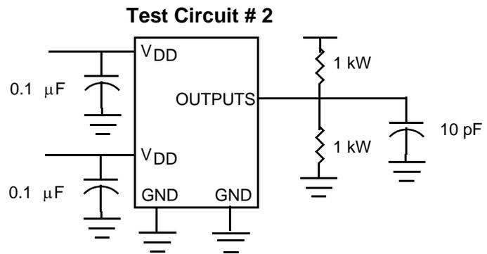
For parameter t8 (output slew rate) on -1H devices
