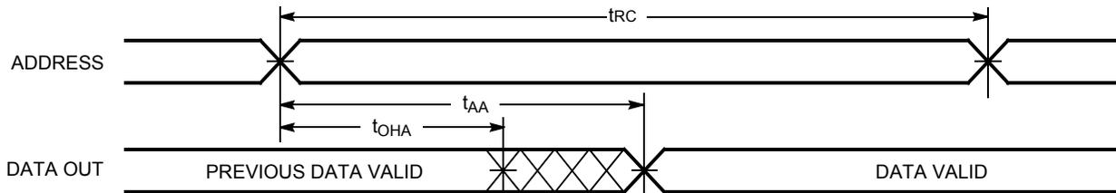
Figure 7. Read Cycle No. 2 ( $\overline{OE}$  Controlled) [20, 21, 22]
