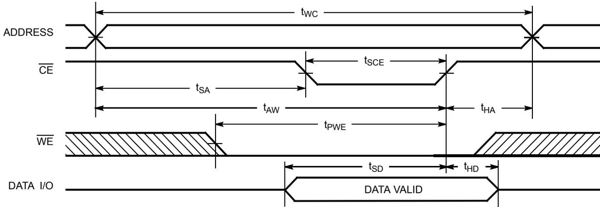
Figure 10. Write Cycle No. 3 ( $\overline{WE}$  Controlled,  $\overline{OE}$  LOW) [27, 30]
