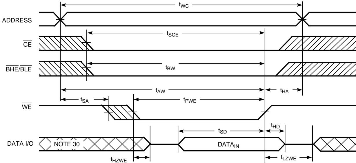
Figure 9. Write Cycle No. 4 ( $\overline{BHE}/\overline{BLE}$  Controlled,  $\overline{OE}$  LOW)<sup>[28, 29]</sup>
