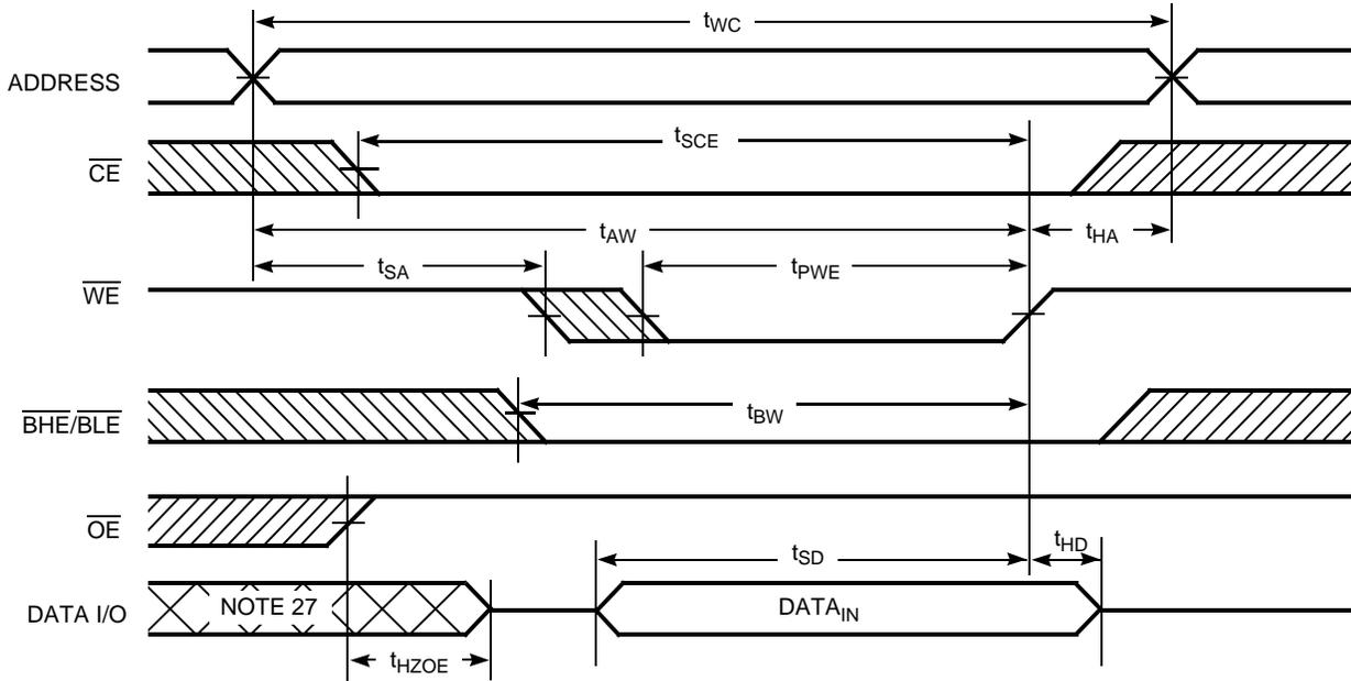
Figure 7. Write Cycle No. 2 ( $\overline{CE}$  Controlled)<sup>[23, 24, 25, 26]</sup>
