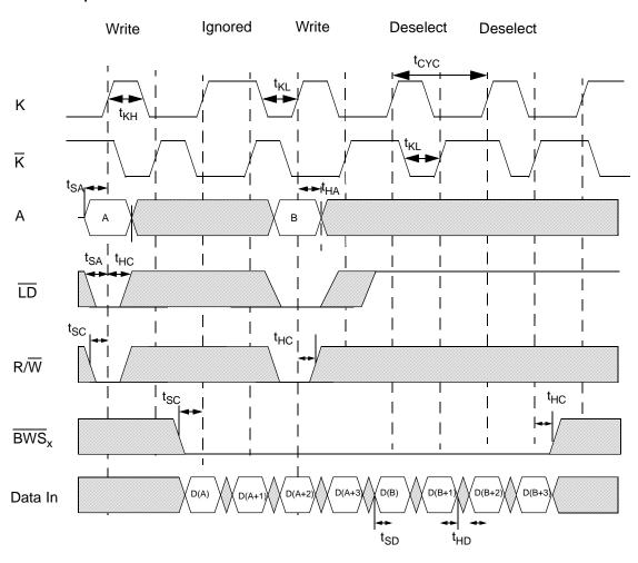
C and  $\overline{C}$  reference to Data Outputs and do not affect Write operations. Activity on the Read Port is unknown.
