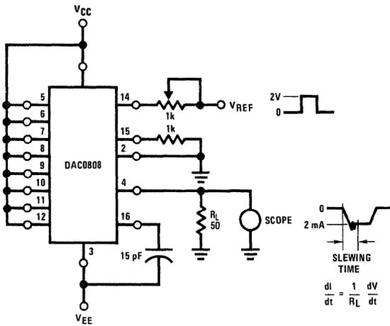
FIGURE 6. Reference Current Slew Rate Measurement (Note 7)
