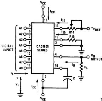
$V_I$  and  $I_1$  apply to inputs A1-A8.
