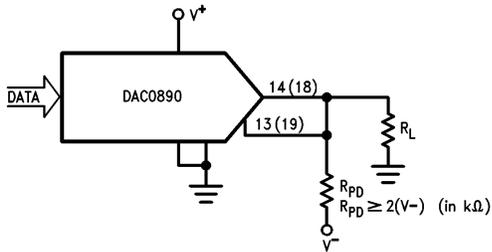
FIGURE 4. Improving Negative Slew Rate
