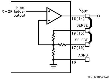
FIGURE 2a. 0V to 2.55V Output Voltage Range
