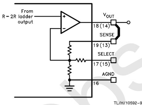
FIGURE 2b. 0V to 10.2V Output Voltage Range
