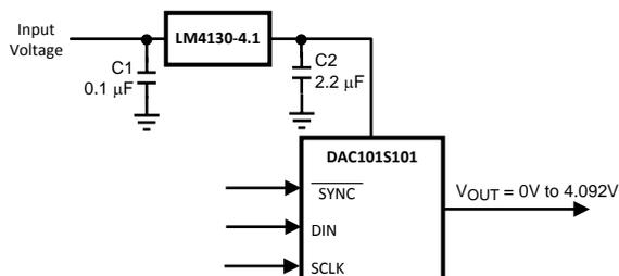
Figure 43. The LM4130 as a power supply
