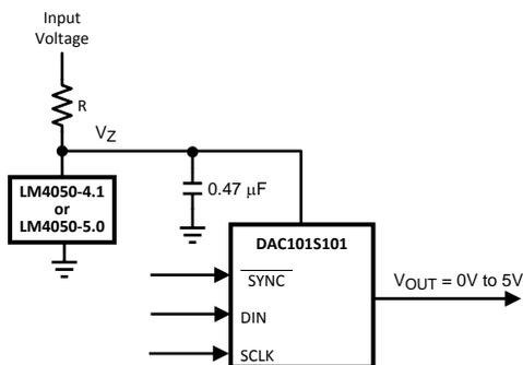
Figure 44. The LM4050 as a power supply
