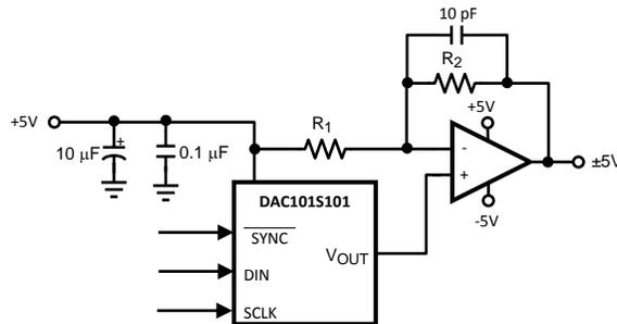
Figure 47. Bipolar Operation
