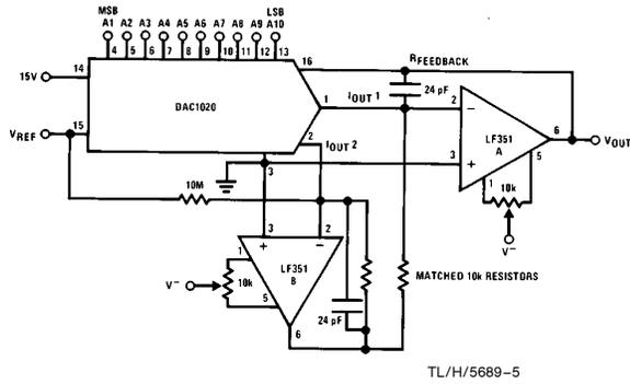
$$V_{OUT} = -V_{REF} \left( \frac{A_1}{2} + \frac{A_2}{4} + \dots + \frac{A_{10}}{1024} - \frac{1}{1024} \right)$$
