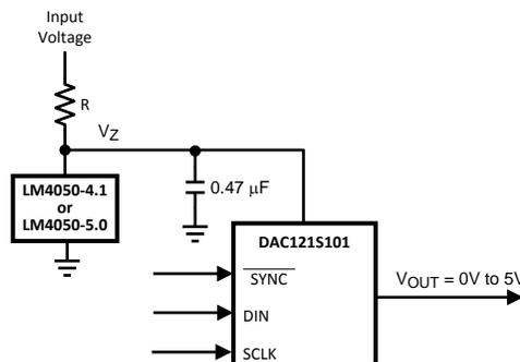
**Figure 40. The LM4050 as a power supply**
