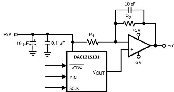
**Figure 43. Bipolar Operation**
