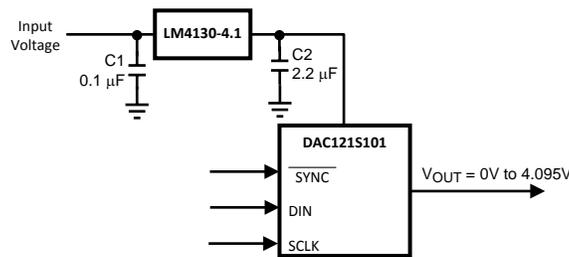
**Figure 39. The LM4130 as a power supply**
