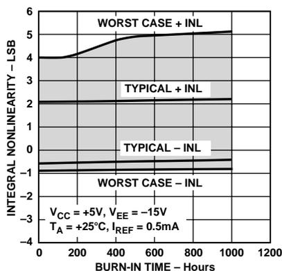
Figure 17. Integral Nonlinearity vs. Time Accelerated by Burn-In
