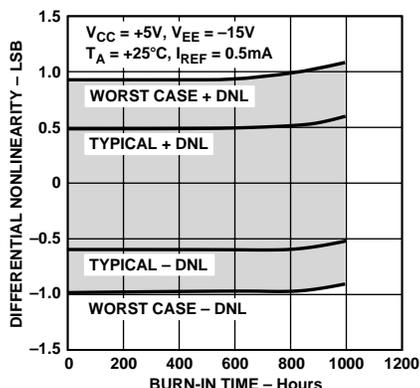
Figure 16. Differential Nonlinearity vs. Time Accelerated by Burn-In
