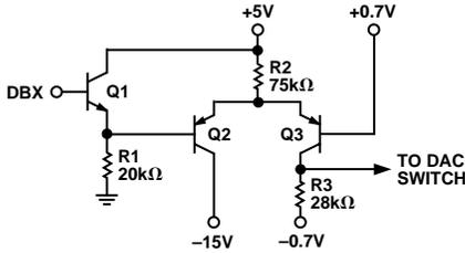
Figure 5. Equivalent Circuit of a DAC16 Digital Input
