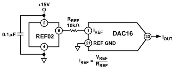
Figure 22. Generating the DAC16's Reference Input Current
