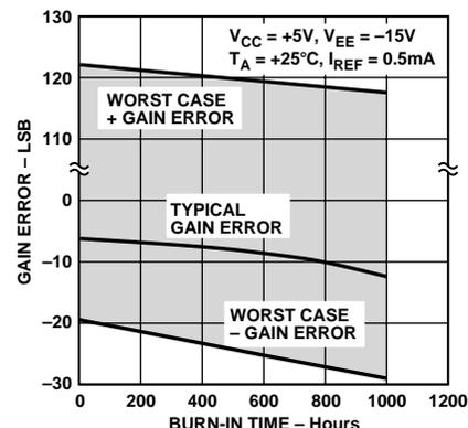
Figure 18. Gain Error vs. Time Accelerated by Burn-In
