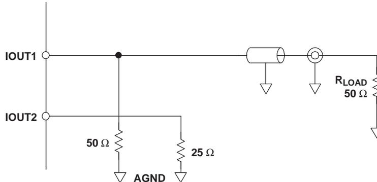
Figure 22. Driving a Doubly Terminated 50- $\Omega$  Cable Using a Single-Ended Output
