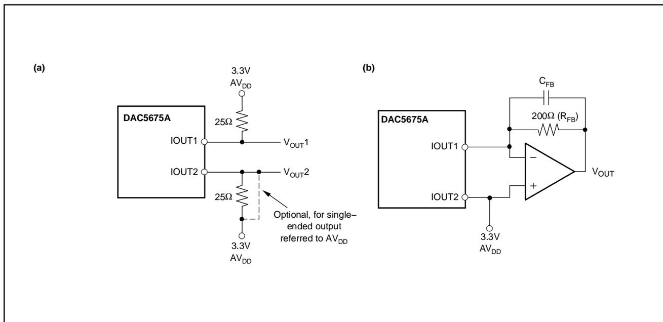
Figure 25. Output Configurations
