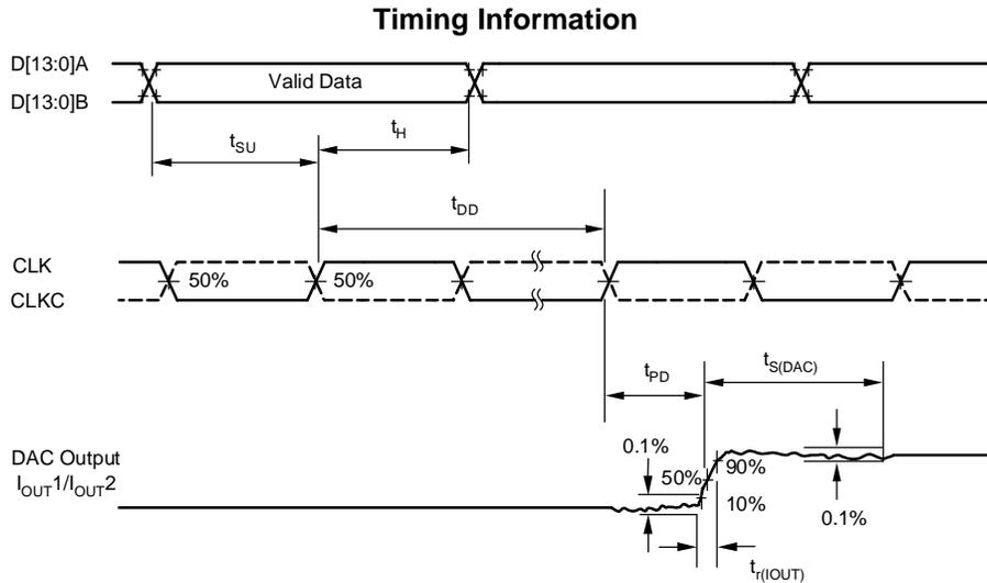
Figure 1. Timing Diagram
