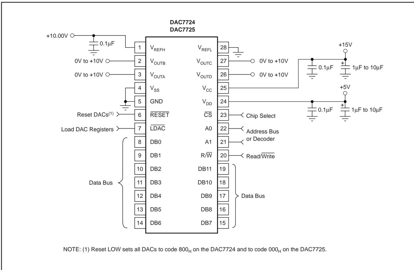
FIGURE 2. Basic Single-Supply Operation of the DAC7724/25.
