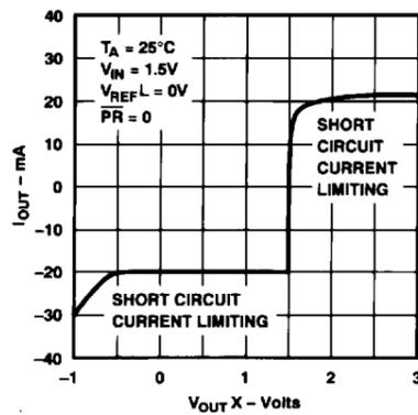
Figure 16. DAC Output Current vs.  $V_{OUTX}$
