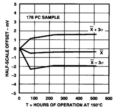
Figure 17. Output Drift Delta Accelerated by Burn-In
