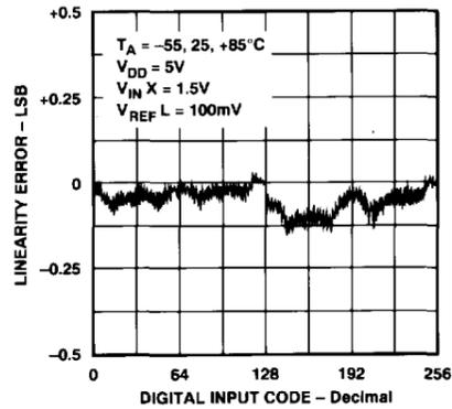
Figure 3. Linearity Error vs. Digital Code vs. Temperature
