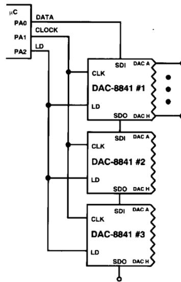
Figure 21. Three-Wire Interface
