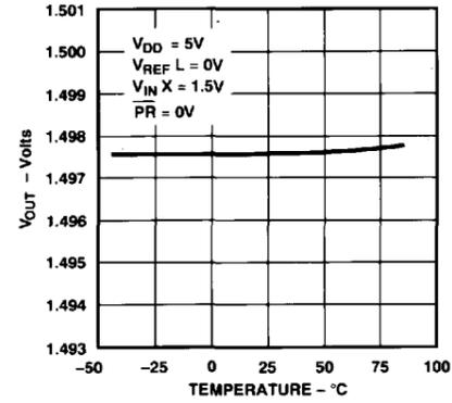
Figure 4. Half Scale vs. Temperature
