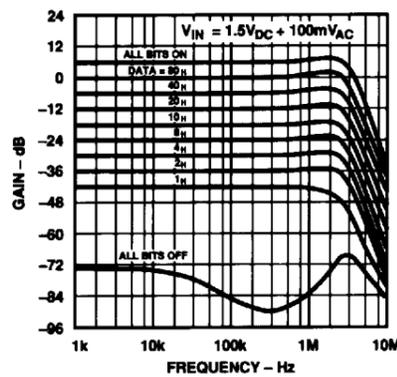
Figure 22. Gain ( $V_{OUT}/V_{IN}$ ) and Feedthrough vs. Frequency
