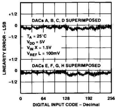
Figure 2. Linearity Error vs. Digital Input Code
