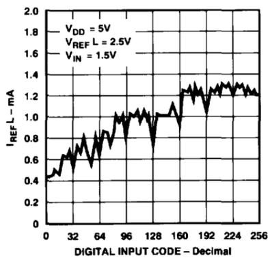
Figure 5.  $I_{REFL}$  Input Current vs. Digital Code
