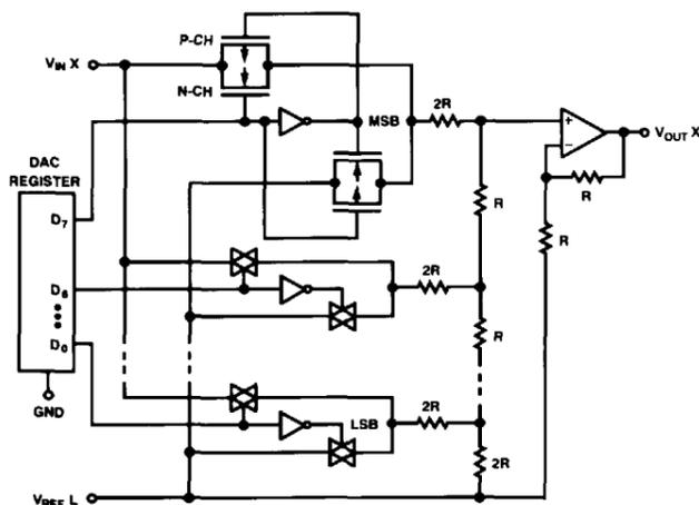
Figure 19. DAC-8841 TrimDAC Equivalent Circuit (One Channel)
