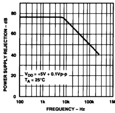
Figure 15. PSRR vs. Frequency
