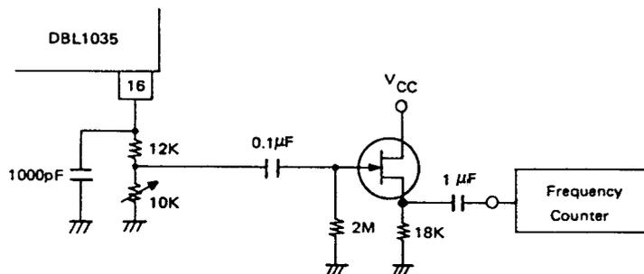
Adjust within 76.00 kHz  $\pm$  50 Hz
