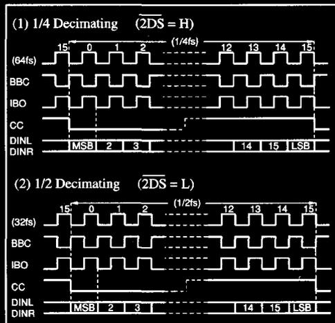
FIGURE 7. ADC Control Signals with  $\overline{\text{IMOD}} = \text{L}$ .
