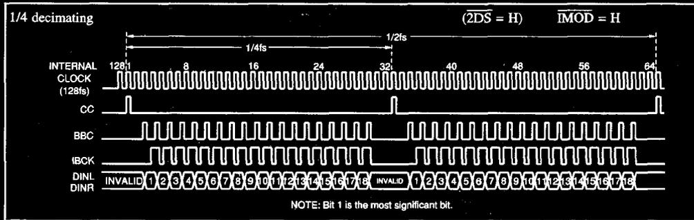
NOTE: Bit 1 is the most significant bit.
