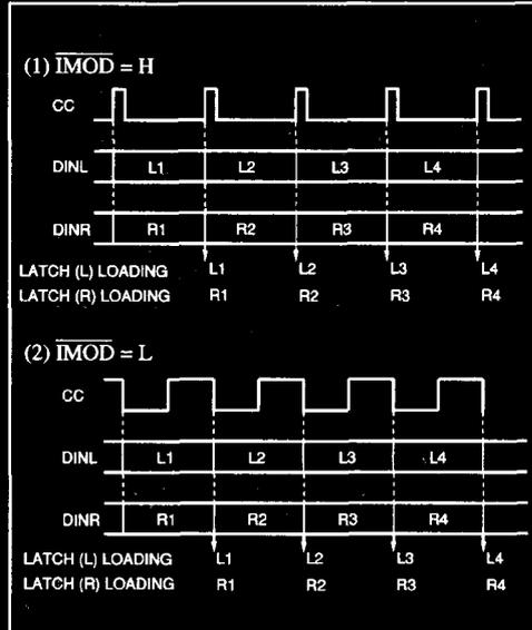
FIGURE 5. Input Data Latch/Loading Timing.
