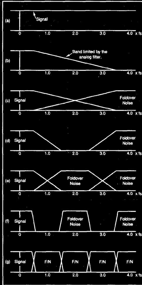
FIGURE 2. The Associated Spectra of the Oversampling-Decimating Technique.
