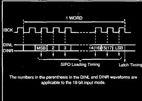
FIGURE 4. SIPO Input Data Loading Timing.
