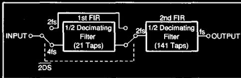
FIGURE 3. Filter Arithmetic Structure
