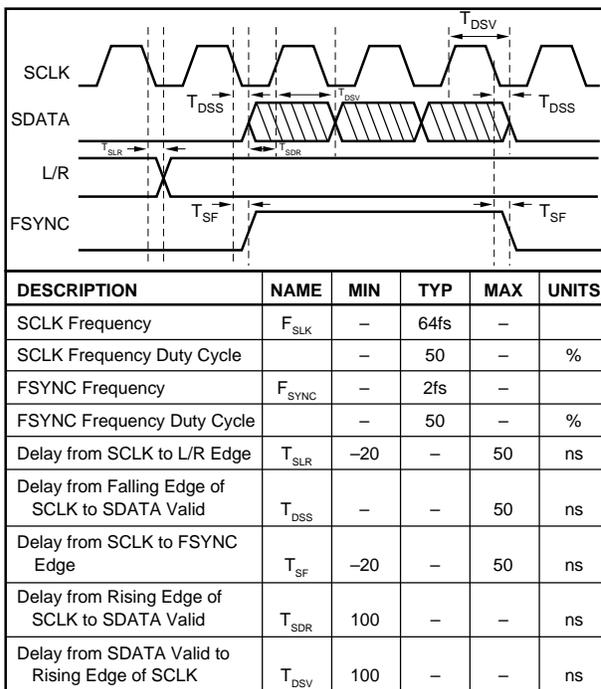
FIGURE 3d. Output Timing of Master Mode, DF1760.
