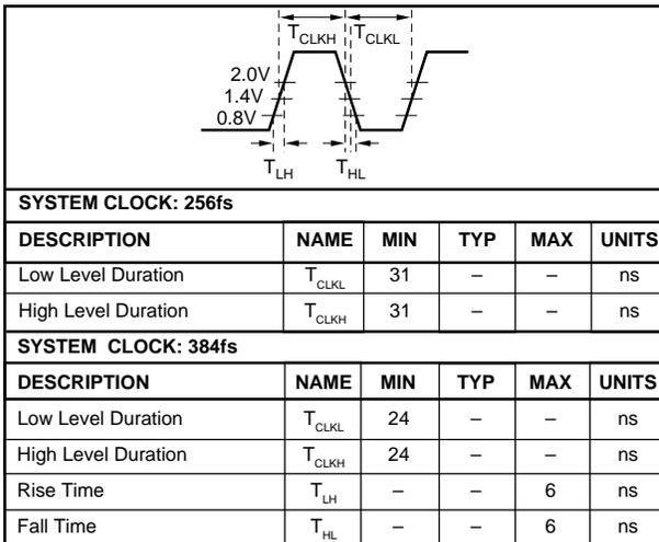
FIGURE 3c. System Clock Timing Requirements of DF1760.
