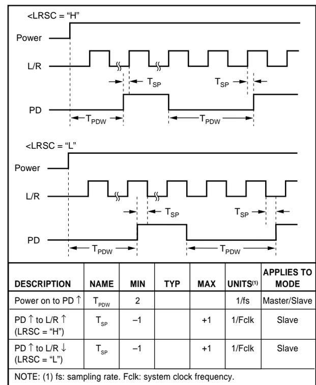
FIGURE 3f. Power On and Mode Reset Timing.
