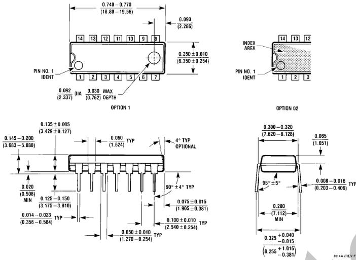
**14-Lead Molded Dual-In-Line Package (N)**
