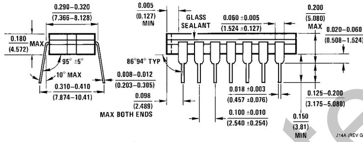
**14-Lead Ceramic Dual-In-Line Package (J)**
