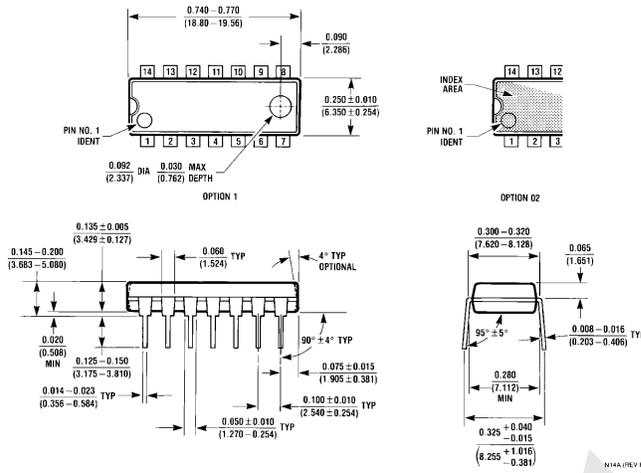
**14-Lead Molded Dual-In-Line Package (N)**
