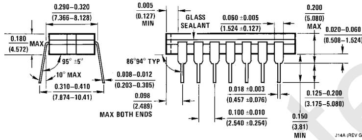
**14-Lead Ceramic Dual-In-Line Package (J)**
