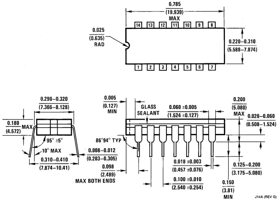
**14-Lead Ceramic Dual-In-Line Package (J)**
