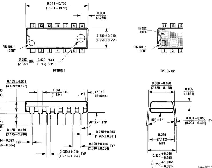
**14-Lead Molded Dual-In-Line Package (N)**
